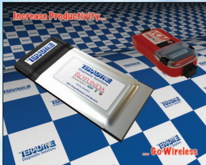
The capability to add Wi-Fi was included in the design when VCM was developed in 2003. In recent surveys one of the top items requested was wireless connectivity for VCM. Based on this input, we developed the new VCM Wireless LAN Module.
