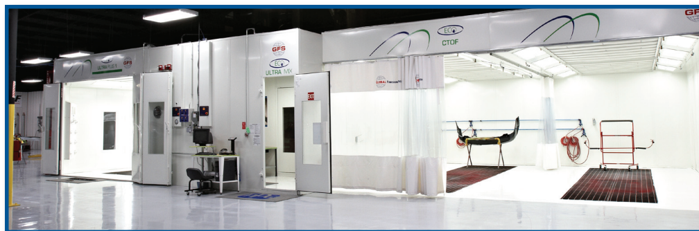
The new 9,400-square-foot Paint and Body Technology Center is a fully equipped bodyshop and includes large eco-friendly paint booths that help determine how paint and adhesives react with newly developed repair procedures.
