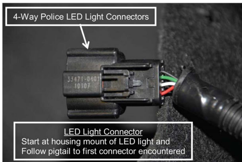
4-Way Connector For All Police LED Light Heads
