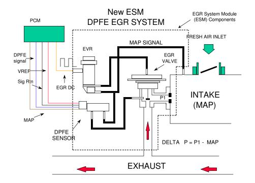
The Delta Pressure Feedback EGR Monitor is a series of electrical tests and functional tests that monitor various aspects of EGR system operation.
