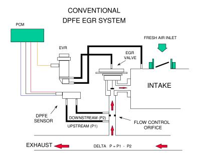
The Delta Pressure Feedback EGR Monitor is a series of electrical tests and functional tests that monitor various aspects of EGR system operation.
