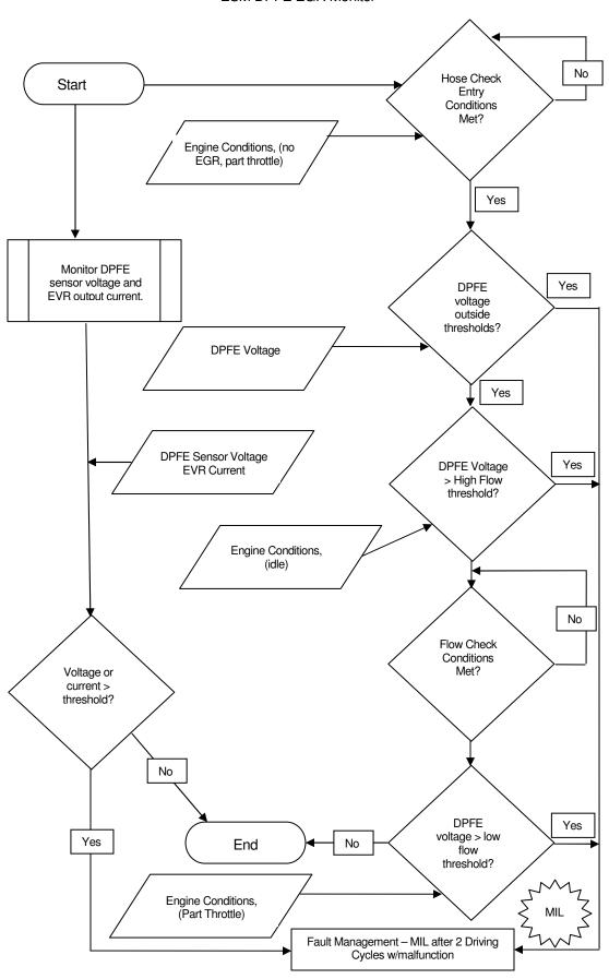
The ESM Delta Pressure Feedback EGR Monitor is a series of electrical tests and functional tests that monitor various aspects of EGR system operation.
