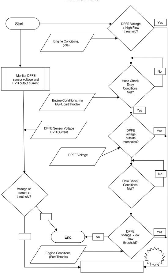
The Delta Pressure Feedback EGR Monitor is a series of electrical tests and functional tests that monitor various aspects of EGR system operation.
