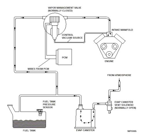
The evap system integrity test is done under conditions that minimize vapor generation and fuel tank pressure changes due to fuel slosh since these could result in false MIL illumination. The check is run after a 6 hour cold engine soak (engine-off timer), during steady highway speeds at ambient air temperatures (inferred by IAT) between 40 and 100 °F.
