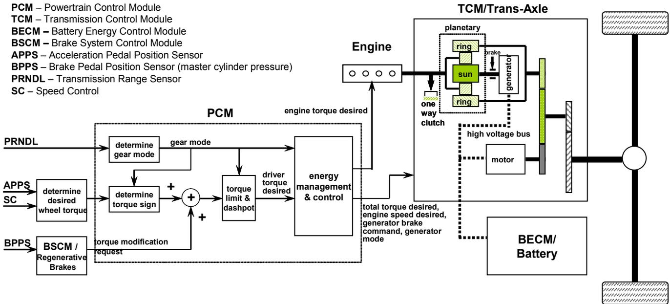
The Hybrid Electric Vehicle Control System uses four modules to control hybrid electric powertrain functions:
