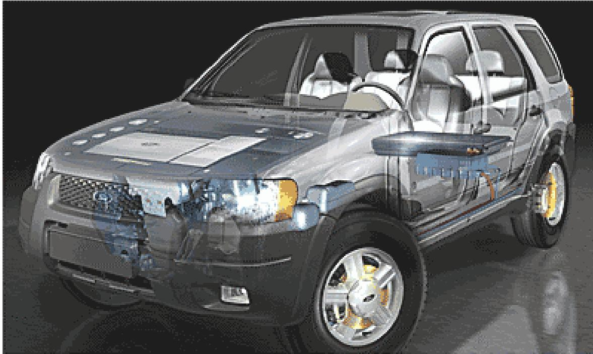
A hybrid electric vehicle is powered by a conventional engine with an electric motor added for enhanced fuel economy and reduced emissions. The electric motor can also be used to boost power and enhance performance (like an extra "charge"). Daily recharging plug-ins aren't needed. This type of vehicle is well suited for the environmentally aware driver who wants better fuel economy and fewer pollutants, but doesn't want the hassle of plug-ins.
