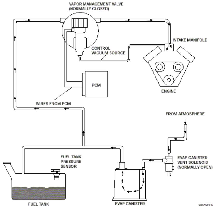
The evap system integrity test is done under two different sets of conditions - first a cruise test is performed to detect 0.040" dia leaks and screen for 0.020" leaks. If a 0.020" dia leak is suspected during the cruise test, an idle test is performed to verify the leak under more restrictive, but reliable, cold-start-idle conditions.
