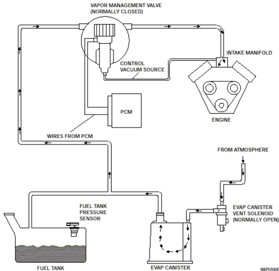
The evap system integrity test is done under conditions that minimize vapor generation and fuel tank pressure changes due to fuel slosh since these could result in false MIL illumination. The check is run after a 6 hour cold engine soak (engine-off timer), during steady highway speeds at ambient air temperatures (inferred by IAT) between 40 and 100 °F.
