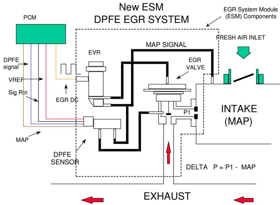
The ESM Delta Pressure Feedback EGR Monitor is a series of electrical tests and functional tests that monitor various aspects of EGR system operation.
