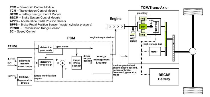
The Hybrid Electric Vehicle Control System uses four modules to control hybrid electric powertrain functions:
