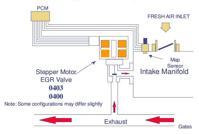
The Stepper Motor EGR Monitor consists of an electrical and functional test that checks the stepper motor and the EGR system for proper flow.
