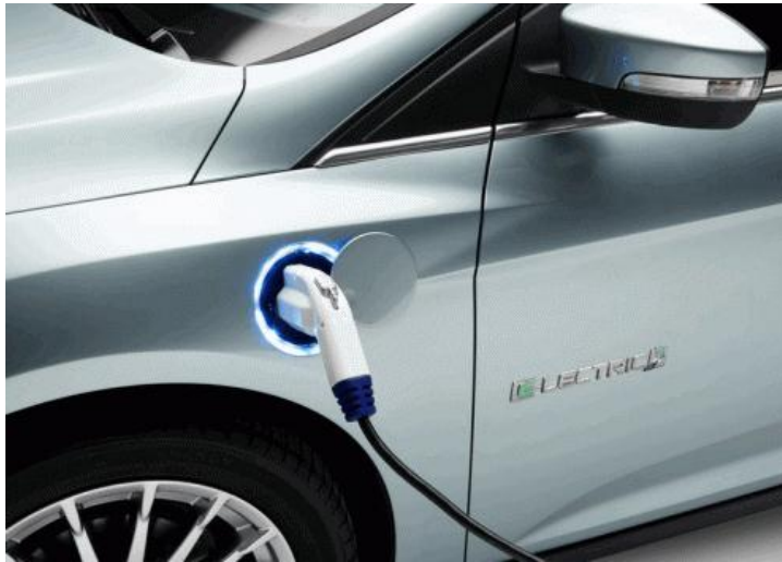
Lighted ring indicates fault and state of charge
