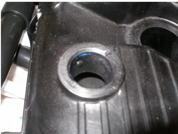
Rocker cover with nub for quarter-turn valve
