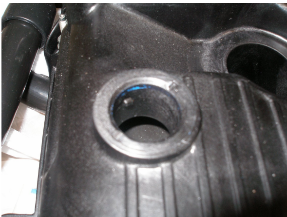
Rocker cover with nub for quarter-turn valve
