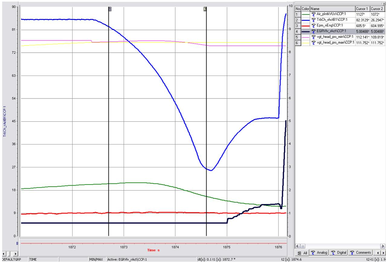
In the example above, at 1871 seconds, the EGR valve is commanded closed, after 3 seconds with EGR off and turbocharger at 85% position, the turbocharger is opened up to 25% position. The 25% position is held for up to 10 seconds. If desired separation of 2kpa at sea level is achieved, the monitor aborts and the test is considered a pass. If desired separation isn't achieved, the monitor remains at 25% position for 10 seconds, and then the test is completed and failed.
