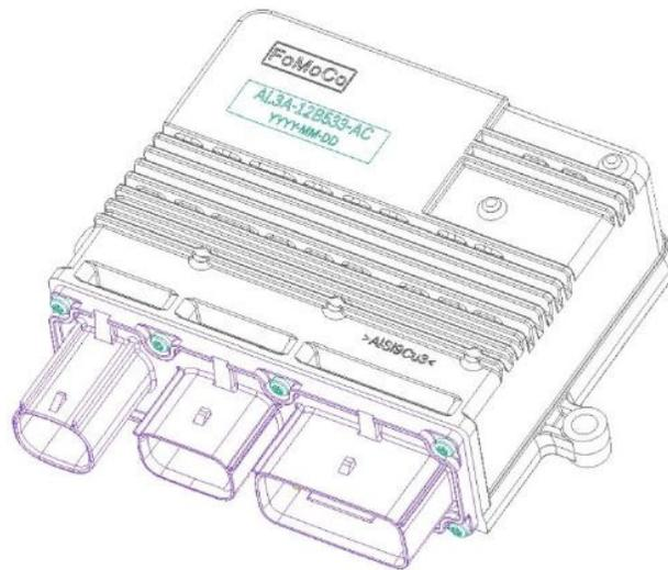
The GPCM is connected to the ECU via Diesel high speed CAN. All data and diagnostics pass over this non-public communication bus. The standard operating voltages for the GPCM are 6.5 volts to 16 volts. Limited operation between 5.5v and 6.5v on the lower range and no operation below 5.5v. Glow function is disabled below 6.5v and above 16.5v.
