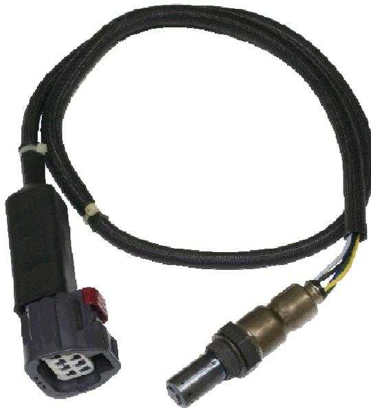
The NOx sensor control module is mounted to the vehicle frame under the body. It is used to control the combination tailpipe NOx and O2 sensor mounted in the diesel aftertreatment exhaust system downstream of the SCR and DPF. It communicates to the ECM via CAN to report NOx and O2 concentrations as well as sensor/controller errors.
