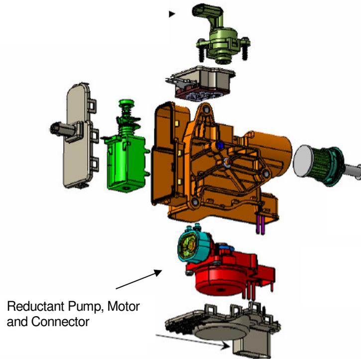
Reductant Pump Motor speed is controlled by a PWM driver in the engine ECU. Increasing the duty cycle of the PWM increases the Pump Motor speed. PWM duty cycles between 87 and 95 are reserved for diagnostics.
