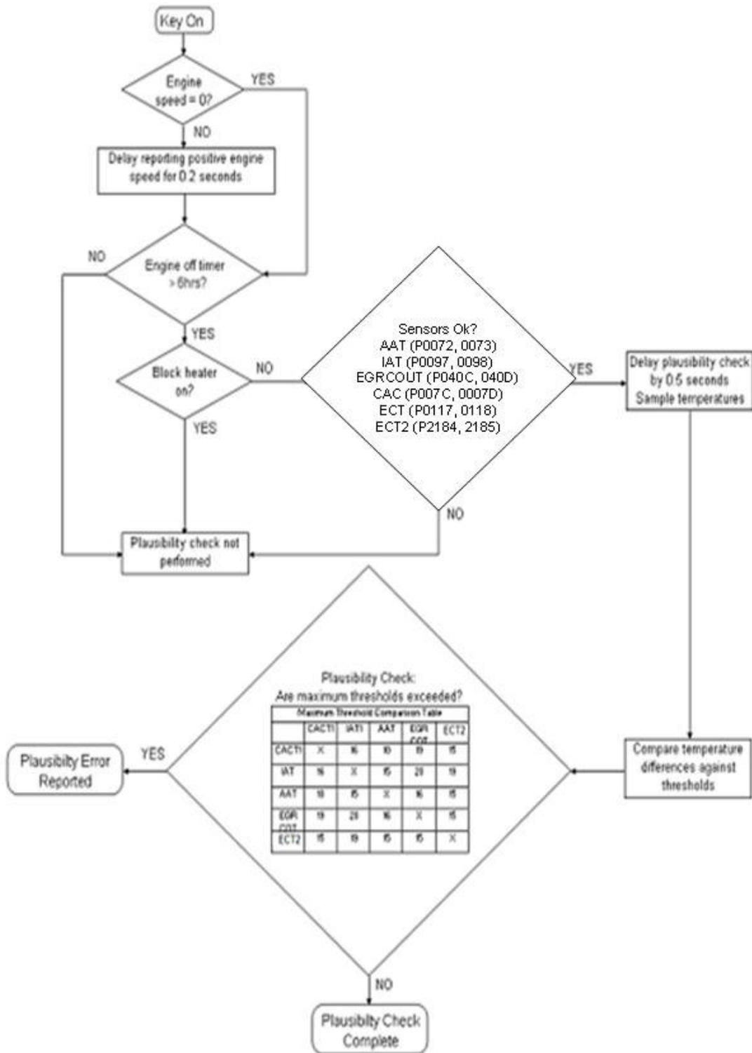
Figure : Air Temperature Plausibility Check Flow Chart
