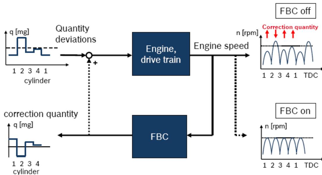
FBC operates in closed-loop control in an engine speed range of 500-1150 rpm, and a commanded injection quantity of 3.5 – 50 mg/stroke. The maximum allowed correction in fuel quantity for an individual cylinder is given by the following table.
