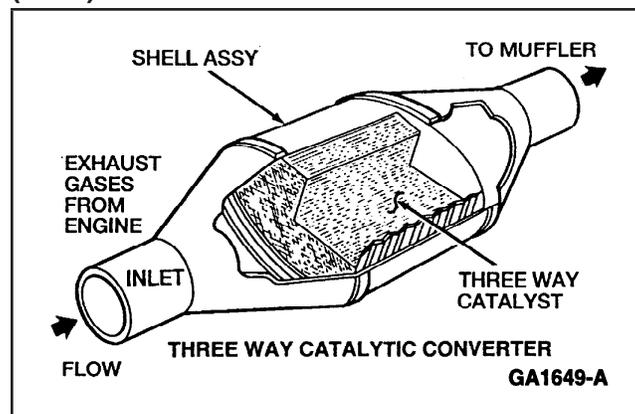
The catalyst metals are thinly coated onto and supported by a honeycomb shaped high temperature ceramic, mounted inside the converter shell. The result is a highly effective converter design having minimum restriction to exhaust gas flow and good durability.
