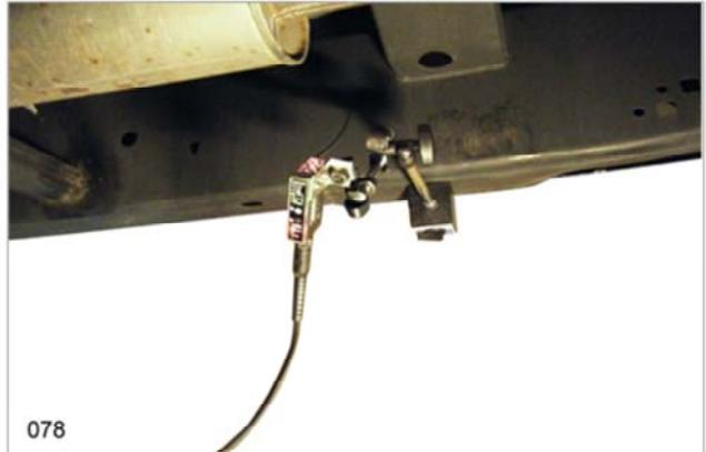
9. Connect the Photo-Tach cable to the Photo-Tach connector on Analyzer.
