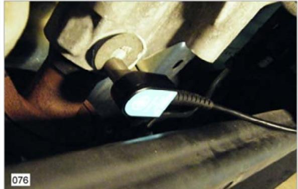
6. Attach the accelerometer to the bottom rear edge of the transmission case (or center support if balancing the rear shaft of a 2 piece driveshaft). Make sure the accelerometer does not rock on the base.
