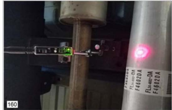
12. Verify Photo-Tach Operation: Rotate the driveshaft to pass the reflective tape through Photo-Tach beam. The green indicator on back of the Photo-Tach will turn on as the tape passes through the beam. See the picture above.
