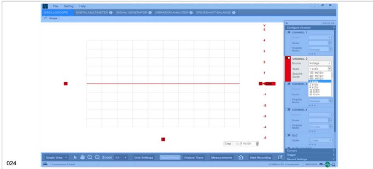
You will see a screen like this when you place a test probe in one of the channel ports to test for voltage.
