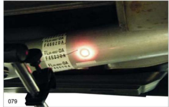
10. Position the Photo-Tach in a location where the beam illuminates the reflective tape. The distance between the Photo-Tach and the driveshaft should be between 6" and 18" (152 to 457 mm).
