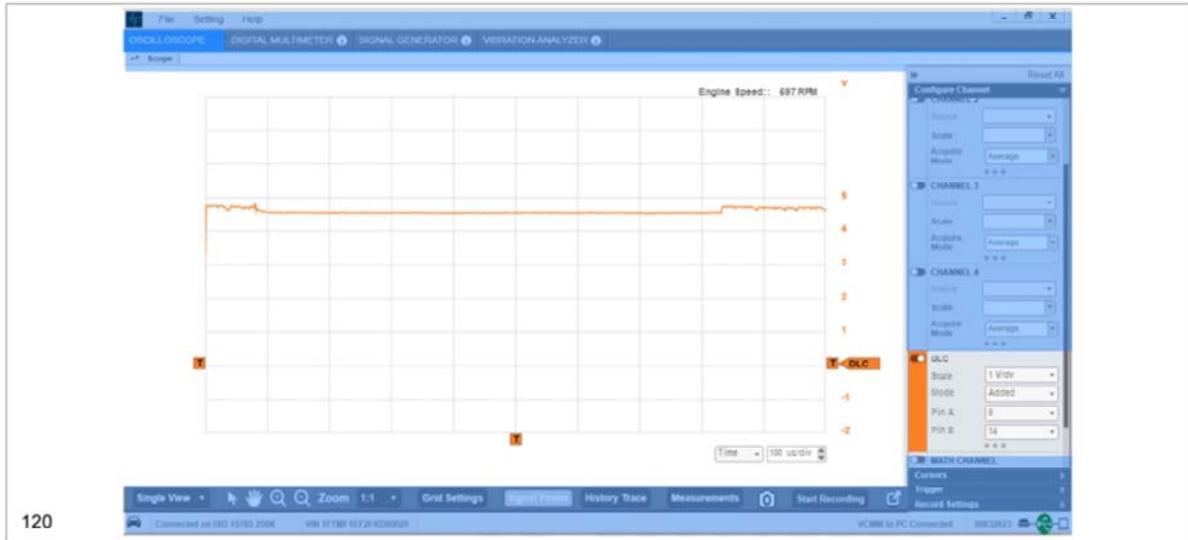
Added mode allows you to monitor the combined voltage of any 2 of the 16 pins in the DLC except pins 4, 5 and 16.
